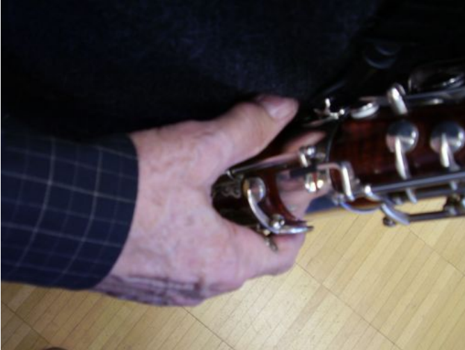
Image 62: guard contacting the index finger above the knuckle. This guard allows Mr. James to keep the index finger from pressing against the C sharp trill key guard.
