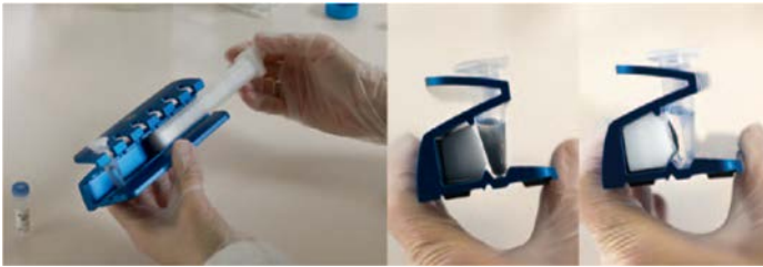
Fig 3.27. The high density of Mag Sepharose beads allows rapid capture by MagRack 6 magnetic device.
